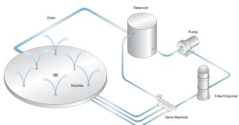
Stand-alone version includes jets, drain, water reservoir, inline chlorinator, filter, valves, pump, and AquaDirector control box. Everything you need excluding piping runs and surfacing material.
