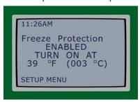
**WARNING:** Freeze Protection will ONLY function with the selector knob in the RUN position. Damage may occur to the user's pool system if Freeze Protection is enabled and the switch is not in the RUN position.
