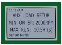
only needs to be powered for 6 hours, the user can set the MAXIMUM RUN TIME.
