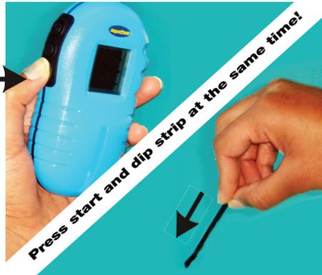
Press start button and dip a strip at the same time. Remove test strip immediately and shake excess water from strip with a simple flick of the wrist.
