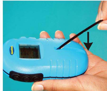
Place tip of strip in back end of channel. Lay flat, pad side down. DO NOT SLIDE THE TEST STRIP ACROSS THE GLASS!
