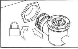
Connect pressure hose with the wall quick connect
