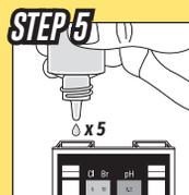
For total chlorine, use the same sample from Step 4 and add 5 drops R-0003. Cap and invert to mix (DO NOT SHAKE).
