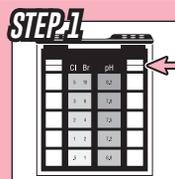
Rinse right comparator test cell and fill with sample water up to black line.
