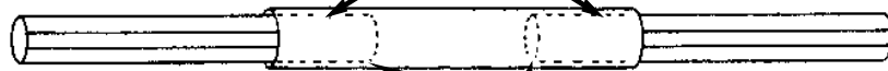
Insert both end tubes equal distance into center tube and mark on center tube where inner tubes end
