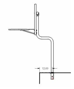
5. The Single Post Basketball units are to be anchored to the deck using a 6-inch deep AS-100D anchor socket or the AS-100P plastic anchor socket, with tightening bolt. Install the anchor in the pool deck 12 inches back from the pool's edge as shown in **FIGURE 5**. Properly bond the anchor socket using the attached bonding screw and the appropriate bonding wire per local codes. Allow concrete to cure before installing Single Post Basketball Unit.
