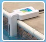
THE POOL SENTRY™ is used to maintain the water level of a pool, spa or pond automatically and unattended. When the Pool Sentry is removed from the box, it is easily assembled by threading the fill tube into the float valve. Snap the fill tube and float valve into the base and fill the base with small rocks or pea gravel. Next, snap the top cover onto the base and attach the garden hose (not included). Finally, adjust the float to the desired position.
