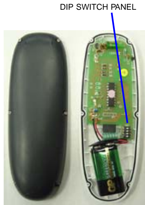
FIG. D TRANSMITTER
