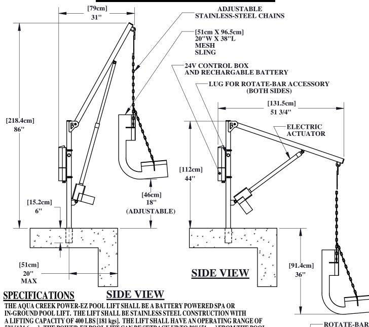
A LIFTING CAPACITY OF 400 LBS [181 kgs]. THE LIFT SHALL HAVE AN OPERATING RANGE OF 53" [134.6 cm]. THE POWER-EZ POOL LIFT CAN BE SETBACK UP TO 20" [51 cm] FROM THE POOL EDGE WITH A 360° MANUAL ROTATION. THE UNIT SHALL INCLUDE A 6" [152 mm] DEEP ANCHOR WITH AN ANTI-TAMPER LID, AND A 20" [51 cm] WIDE BY 38" [96.5 cm] LONG MESH SLING. THE UNIT IS PORTABLE AND CAN BE REMOVED WITHOUT TOOLS. A  $\phi$ 1" ROTATE-BAR IS INCLUDED TO HELP ROTATE THE LIFT. A LIMITED LIFETIME WARRANTY IS STANDARD.
