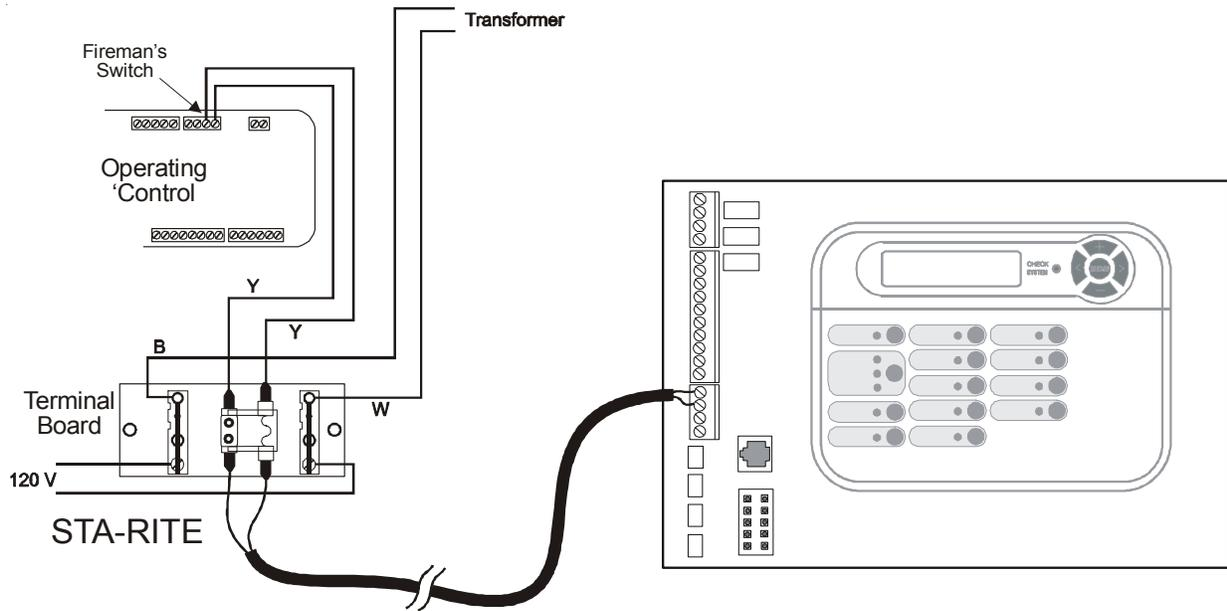
**Hayward Variable Speed Filter Pump:** Refer to the diagram below for proper low voltage communication wiring between the Pro Logic and the Hayward Tristar Variable Speed Control (VSC).
