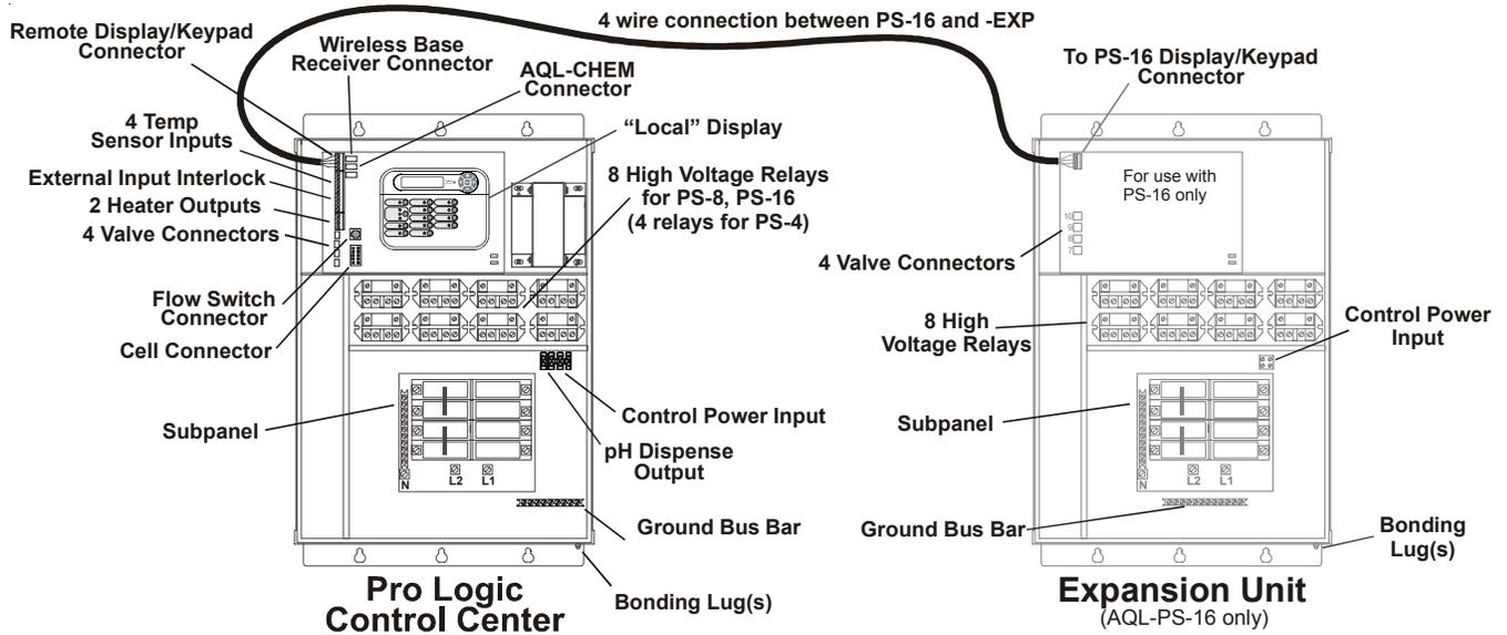
The Pro Logic Control Center and PS-16 Expansion Unit require both high and low voltage connections. Low voltage connections will be made to actuators, sensors, remote keypad, etc. High voltage connections will be made to pumps, lights, etc., as well as providing direct input power to the Control Center. Always:
