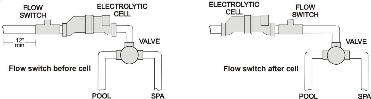
The cell may be mounted vertically or horizontally, and water can move in either direction through the cell. Install using the 2" unions provided in the P-KIT purchased separately. Tighten unions **BY HAND** for a watertight seal. For systems with 1½" plumbing use adaptors (provided by installer).
