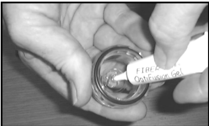
6. Fill Standard Lens reservoir with gel. (No gel required in Wide Angle Lens.)
