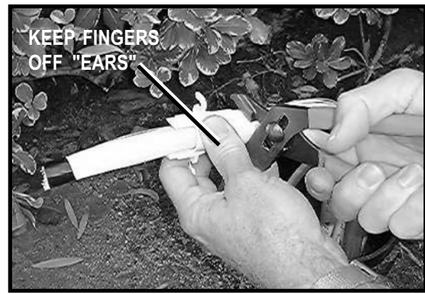
4. Securely tighten the ferrule assembly.
