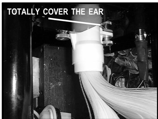
12. Tip PG2000 back and secure "ears" under thumbscrews.
