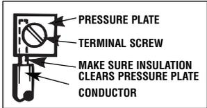
4. Follow wiring diagram on page 4 of this manual and make LINE and LOAD (Pump) connections as shown. Wiring the Freeze Control, first identify each lead by its color (Line: **Black** and **Red**, LOAD: **Blue** and **Yellow**), then make wire connections by using twist on wire connectors.
