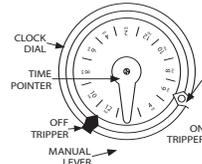
**1. TO SET "ON" AND "OFF" TIMES:** Hold TRIPPERS against edge of CLOCK-DIAL, pointing to time (AM or PM) when ON and OFF operations are desired. Tighten tripper screws firmly.
