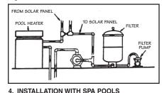
Connect suction side of the booster pump before spa bypass valve, if your pool is plumbed for a spa pool. (See Figure 3). Figure 3: Installation with Pool/Spa Combo
