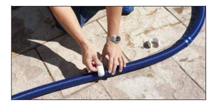
3. Place the **hose weight (#17)** on the hose. You will need one hose weight if your pool depth is less than 8 feet, two if the pool depth is more.
