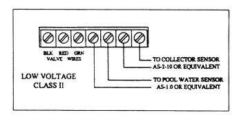
At the termination of all sensors, weather insulating procedures should be exercised. Wire nuts should be sealed with silicone.
