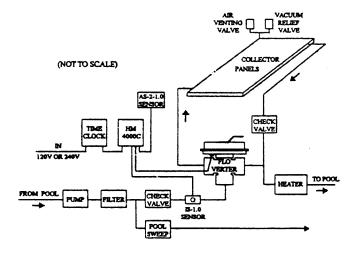
The valve diverter is pre-drilled with a small bypass hole which allows the collector to drain when the pump is off or when collection is not diverted through the collector. Install a check valve as shown in illustration. The check valve prevents water from the solar collectors passing backward through the filter into the pool when the pump is off.
