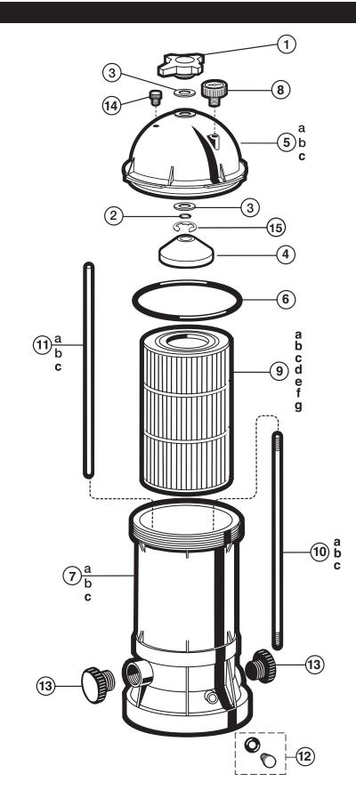
StarClear<sup>®</sup> Plus CARTRIDGE FILTER SERIES AND SEPARATION TANK REPLACEMENT PARTS
