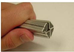
While holding the ferrules together, insert into the strain relief opening as illustrated.
