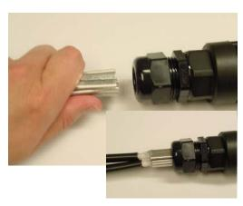
Gently push all the ferrules until it is completely inside the strain relief and cannot not be pushed any farther. Now **HAND** tighten the strain relief to hold the ferrules and fiber in place.
