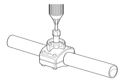
9. Insert the flow diverter into the clamp assembly and snap it into place. Snap the outer housing onto the clamp assembly.
