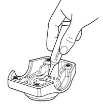
7. Install your Nature<sup>2</sup> Express on schedule 40 PVC pipe only. Failure to heed this warning can result in equipment failure. Position the clamp assembly on the pipe, with the arrow pointing in the direction of the flow of water and hand tighten the nuts and bolts. Tighten nuts an additional 1/4 turn using a wrench or socket. Do not over-tighten.
