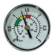
**1,3 kg/cm²** - **18,5 PSI:** The pressure is 0.5 kg/cm² more than the initial pressure, indicating that WASHING is required.
