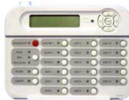
Shown below is a labeled remote control to a Pro Logic PS pool control. Note that labels have been placed over the generic names to make the keys human readable. In this case, the Pool Filter, Gas Heater, Spa Filter and Water Feature are all turned on.
