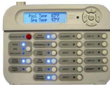
The menus are mainly used to configure the pool and change temperature setpoints. Most user interaction is via the direct-access keys in the lower half of the control.
