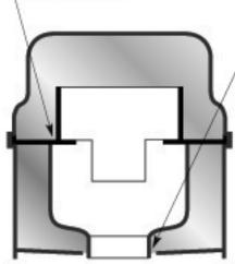
Air intake at bottom of the Silencer™ creates a tortuous path, trapping noise inside the blower.
