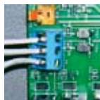
Figure 1. Remote Pool-Off-Spa Connection (3-Wire Connection)
