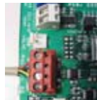
Figure 3. AquaLink RS 485 Communication (4-Wire Connection)
