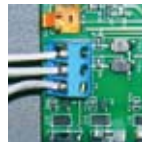
Figure 1. Remote Pool-Off-Spa Connection (3-Wire Connection)
