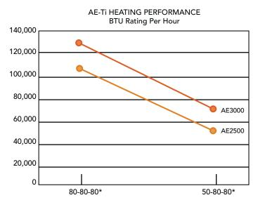
${}^\star\!\text{Air}$  temperature, water temperature and relative humidity at 50 GPM
