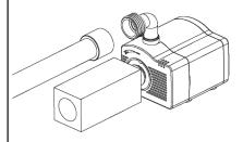
A 1/2" Barbed fitting is also provided that can be used instead of the hose fitting. It will fit a 1/2" ID tubing.
