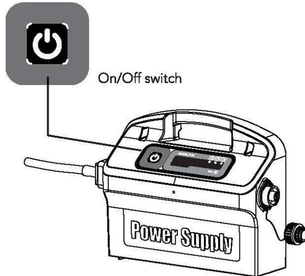
When the power supply is switched on, the 3 LEDs will blink for 5 seconds. At this time by pressing the SELECT button you may choose a pool cleaning schedule for the coming week.
