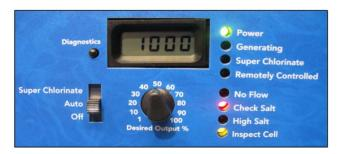
NOTE: Check Salt & Inspect Cell LED's will also be ON if the control is set for the wrong Turbo Cell type or the cell is unplugged.
