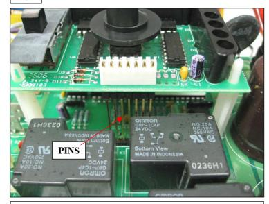
Remove and/or reseat DSP board. Pins may be shorted together or not making contact with connector. If pins are good, check for 3 to 5 volts (DC) on pins 1 & 3, starting from the left. If DC voltage is correct, replace DSP board.
