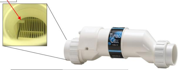
LCD display will read "COLD" when the water temperature is below  $50^{\circ}$  F LCD display will read "HOT" when the water temperature is above 140  $^{\circ}$  F If the water temperature reads 215  $^{\circ}$  F, the cell temperature sensor is shorted and the cell needs to be replaced.
