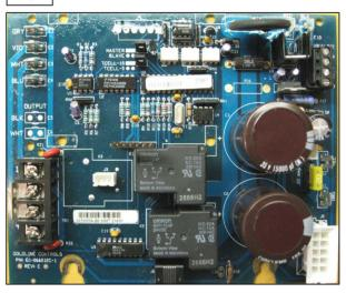
Visually inspect main PCB board for any damaged or burnt components. If damaged or burned, replace the main PCB.
