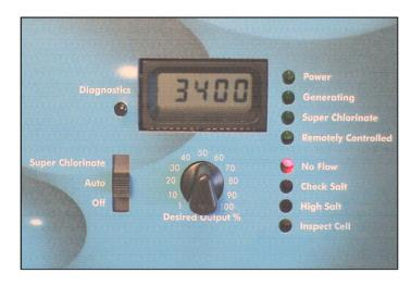
If LED is flashing, wait 60 seconds after starting filter pump. Check for possible turbulence inside of flow T. Installation requires 12 inches of straight pipe before flow switch. There should be no elbow after the flow switch.
