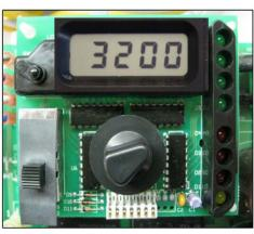
Jumpers on terminal TB1 are configured for 240 VAC (factory default), but there is 120 VAC applied to control box.
