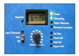
To switch Cell Type, cycle Main Switch from AUTO → Super Chlorinate → AUTO.
