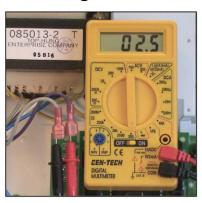
Insert probes and measure resistance between the Blue & White wires and the Violet & Gray wires.
