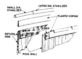
Make a return hem as illustrated. DO NOT cut off excess liner material as the liner will "Slip" from under the plastic coping, causing liner to fall back into the pool. Smooth liner against wall and secure to top of wall with plastic coping. Place stabilizer rails over coping, alternately telescoping small diameter into large diameter about 6 inches as before. One large diameter stabilizer rail fits between each pair of side supports. They DO NOT telescope.
