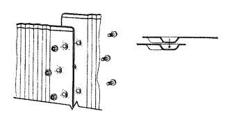
If interlocking wall ends do not meet, adjust all vertical end caps in or out uniformly as required. Do not make the total adjustment with only one or two vertical end caps. Fasten wall with screws supplied in wall carton. Screw head must be on the inside of pool. When finished, go back and retighten all screws and nuts. Remove any burrs on all screw heads. Place protective vinyl strip, included in hardware pack, over screw heads and tape in place.
