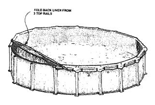
With the help of two or three people, raise and hold the liner up from any three top rail sections. Remove four top connectors, three top rails and two vertical end caps. REMEMBER, NEVER ALLOW LINER TO FALL BACK INTO POOL.
