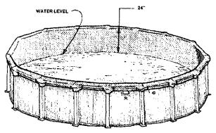
Continue filling pool. Never allow liner to fall back into pool. Water between the liner and wall can cause pool failure. When pool has approximately 24 inches of water, stop filling. DO NOT resume until Steps 15, 16, and 17 are completed. CAUTION: Do not cut any openings into liner at this time.
