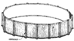
Carefully follow details shown below to assemble verticals to pool, use exploded view for your pool. Use all necessary hardware. Refer to parts list for correct screw locations. Check pool for roundness by measuring across the pool from side to side. Pool diameter should be the same from point to point.
