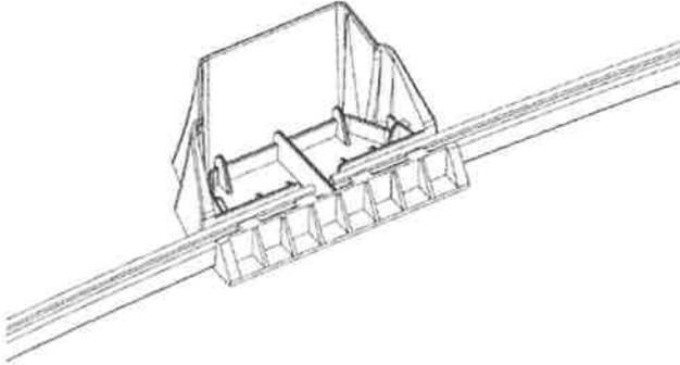
Assemble all bottom tracks to the bottom plates to form a perfect circle with a diameter and a radius in accordance to the chart
