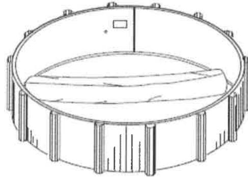
Carefully unfold the liner (U-Bead or Overlap), bringing the bottom-sidewall seam close to the wall base. Make sure the side with the protruding seam faces downward or that the patterned side faces upward.
