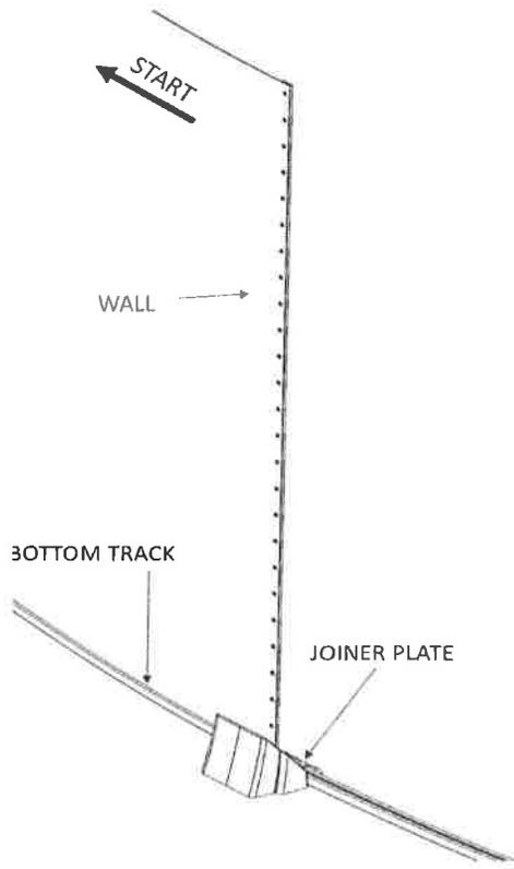
Begin inserting the wall into the bottom wall tracks in the middle of a joiner plate. At first, the wall should be kept in place with one or two support bars (or extra persons). One person should uncoil the wall on a beam or a plank while a second person inserts it in the bottom wall tracks. Do not uncoil more than 3 m (10') of wall before you install a support bar to reinforce the structure.
