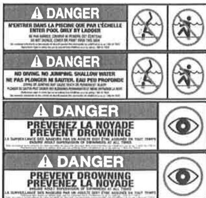
Install a minimum of three (3) safety labels (supplied with the liner) inside the pool so that at least one label is visible no matter where the bather enters the water (See drawing for positioning).
