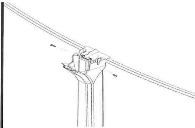
Install the joiner plates on top of each upright then install metal screws at the top of the support posts, making sure the support posts are perpendicular to the ground.
