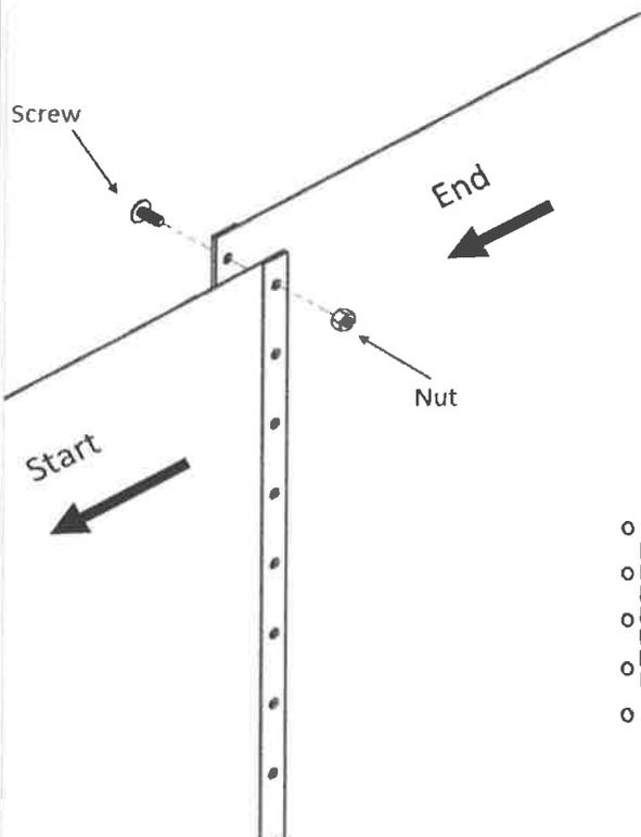
For proper grounding we suggest grounding the second wall bolt from the top of the wall seam. Use a 6 Gauge terminal and a 6 Gauge ground copper wire. Connect the wire to a 36" (1 m) grounding rod that will be inserted into the ground at least 36" (1 m) from the pool's perimeter. Please check the local electrical grounding codes for above ground pools in your county or state, as it varies from state to state.
