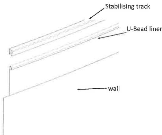
Hang the "U-Bead" liner on the top of the wall and install the round stabilisers to secure.
