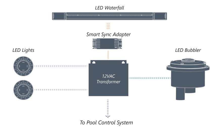
Integrate with all other pool lighting with no special requirements. Simply connect the same as any other LED pool lighting. One line per component connects to a 12VAC pool transformer. All Smart Sync products connected to the same transformer will synchronize. Connect the transformer to pool controls for complete system integration.
