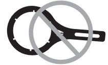
DO NOT USE CAP TOOL TO TIGHTEN CAP. Use for removal only.
