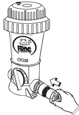
Insert reducer bushing into male adapter on both sides in place 5 to 10 seconds to bond.
