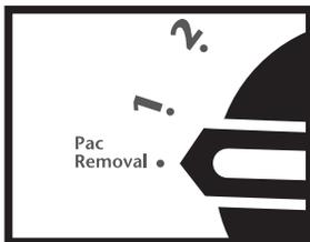
Turn off pump. Turn dial to Pac Removal. This reduces the flow of water into the unit when the cap is open.
