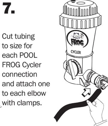
Cut tubing to size for each POOL FROG CYCLER connection and attach one to each elbow with clamps.
