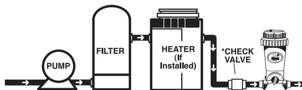
To prevent damage to heaters or filters, see your dealer about installing a **corrosion resistant check valve** which will reduce the back flow of chlorine gas when the Cyclor is turned off.
