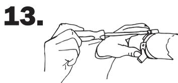
Tighten scoop clamps with a screwdriver.
