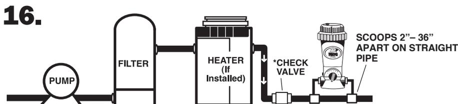
To prevent damage to heaters or filters, see your dealer about installing a **corrosion resistant check valve** which will reduce the back flow of chlorine gas when the Cyclor is turned off.
