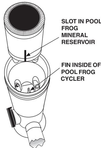
Find slot on side of POOL FROG Mineral Reservoir and line up with fin inside the POOL FROG Cycler. Lower POOL FROG Mineral Reservoir into POOL FROG Cycler until secure.
