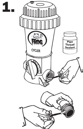
Following pipe thread sealant directions, brush sealant onto POOL FROG Cyclor threads in both ports and on both male adapters.
