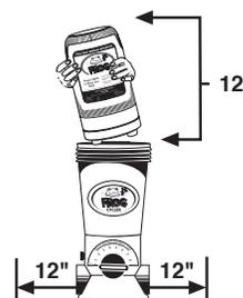
Allow a minimum of 12" above and on each side of POOL FROG Cyclor to ensure room for easy replacement of POOL FROG Mineral Reservoir and POOL FROG Bac Pac.
