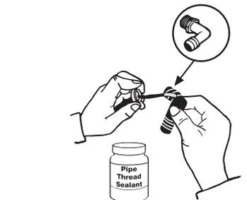
Following pipe thread sealant directions, brush sealant onto elbow threads.
