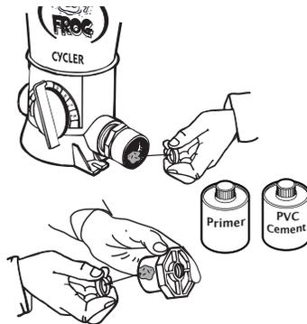
Following Primer directions, brush Primer on reducer bushings and inside of male adapters. Repeat this process with PVC cement following manufacturer's directions on that product.
