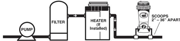
The POOL FROG Cyclor should always be installed between the filter and pool (or between heater and pool if applicable). Never install POOL FROG Cyclor before the heater or damage to the heater could occur.
