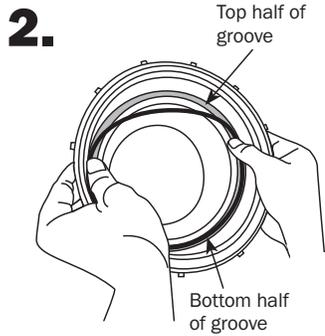
Place new O-ring in bottom half of groove.
