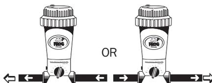
Do NOT install this POOL FROG Cyclor in either flow direction. Bi-flow valve design allows installation in either flow direction.
