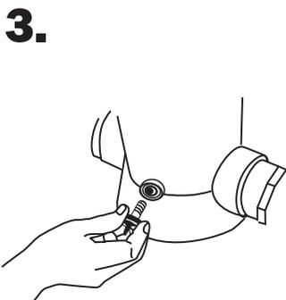
Unscrew knob in the back of POOL FROG Cycler. Allow all water to drain.
