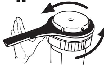
Open POOL FROG Cycler Cap. Use the cap tool included with POOL FROG Cycler to loosen cycler cap by hitting the handle with the flat of your hand counter clockwise.
