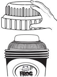
Turn pump off. Turn control dial to Pac Removal. Remove cap from POOL FROG Cycler and stand back to let any chlorine fumes dissipate.
