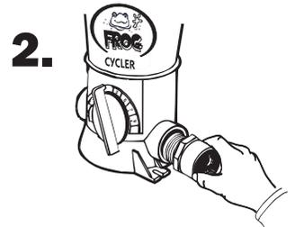
Screw a male adapter into each port of POOL FROG Cyclor and hand tighten.
