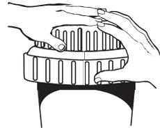
Replace cap by hand only. DO NOT OVER TIGHTEN.
