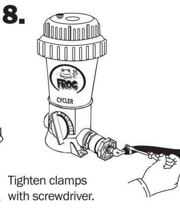
Tighten clamps with screwdriver.
