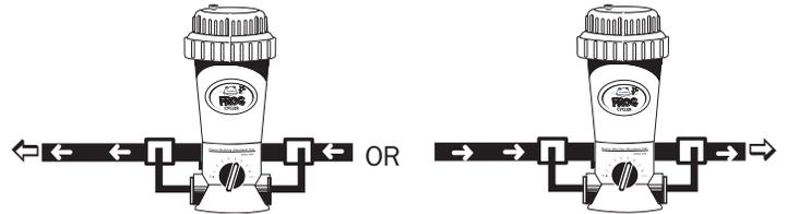
Bi-flow valve design allows installation in either flow direction.
