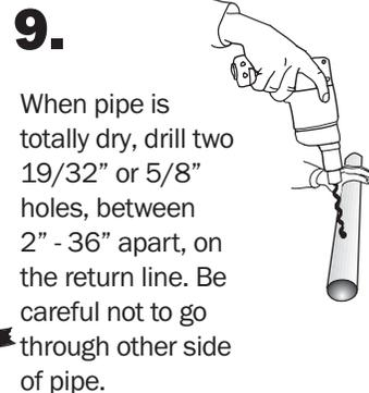
When pipe is totally dry, drill two 19/32" or 5/8" holes, between 2" - 36" apart, on the return line. Be careful not to go through other side of pipe.
