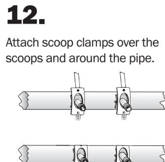
Attach scoop clamps over the scoops and around the pipe.
