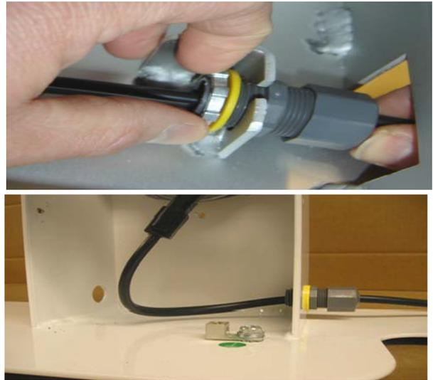
6. Plug motor harness into the connector plug at the motor assembly.
