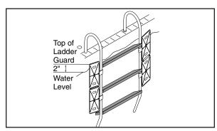
3. Insert the screw through the hole in the ladder guard and into the "U" clamp. Tighten only enough to secure the guard to the ladder rail.
