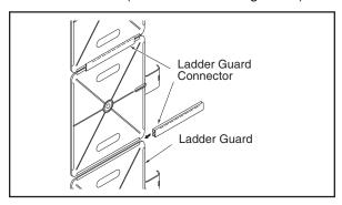
5. Attach two ladder guards underneath the bottom rung by following the same procedure as outlined previously for the side rails.
