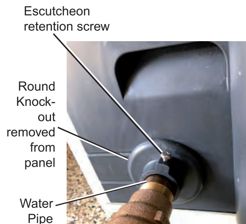
Figure 2. Escutcheon installed on Pressure Relief Valve water pipe (if installed). Be sure the escutcheon covers the circular opening in heater panel.
