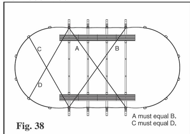
The following are detailed diagrams for every size oval pool that we make. Most of these measurements apply to both the Traditional Buttress oval assemblies and the Buttress-Free oval assemblies. Please use the diagram that applies to your pool to make sure you have everything in its proper position before proceeding with these instructions. Taking a few minutes to check these measurements now can save you major time and efforts down the road if something is not correct.
