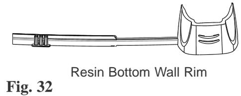
**\* IMPORTANT: Make sure you are using the bottom rails and not the inner stabilizer bars. The bottom rails on some pool models are made of resin and not metal (see Fig. 31 and Fig. 32). The stabilizer bars are always metal and they have male and female end. The bottom rails are the larger width rails that have the straight cuts on both ends. The bottom rails do not interlock (see Fig. 30).**
