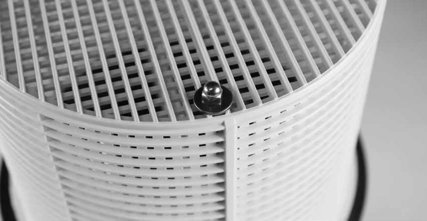
The washer and acorn nut should now rest on the bottom of the basket. If you added the second flange for larger baskets, be sure to keep the slots aligned. *(If your all thread rods are too short to reach, you will need to use the 2 longer all thread rods.)*
