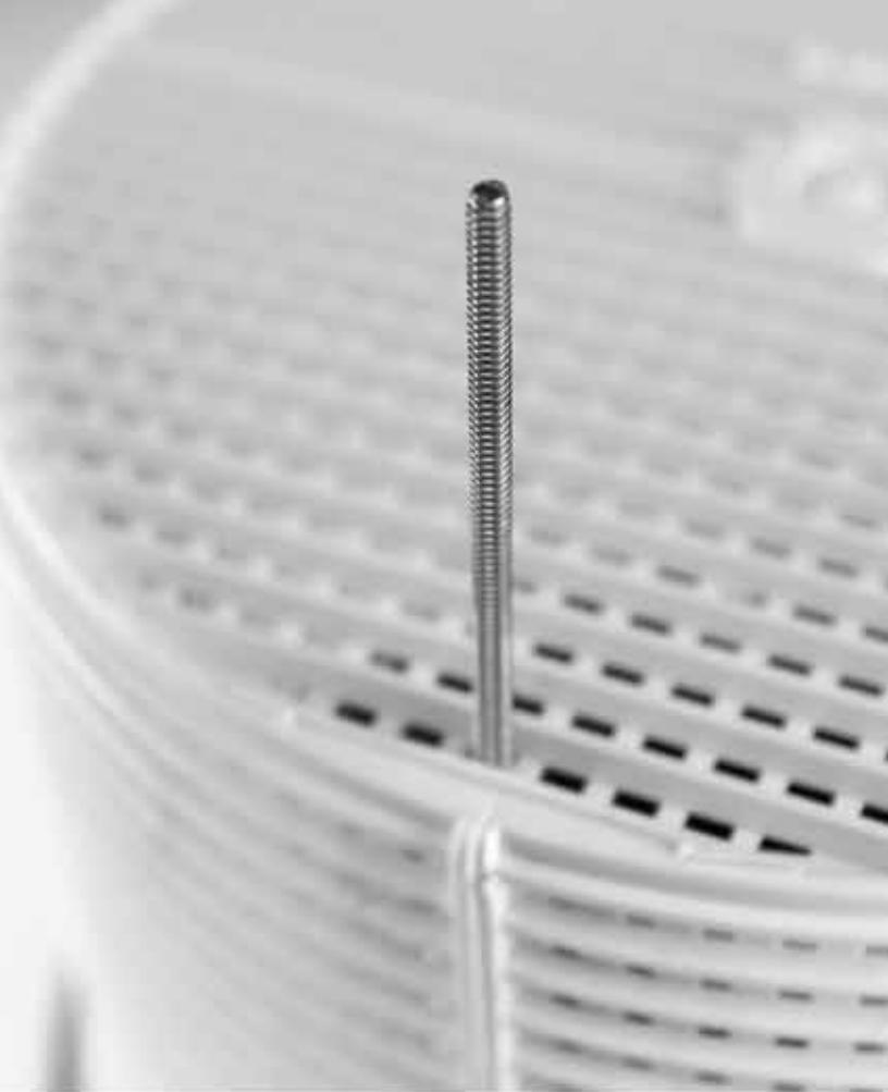
Stand one of the short all threads rods next to the basket vertically, if the rods are taller than the basket, you will use the shorter rods. If the basket is taller than the shorter rods, you will use the longer rods.
