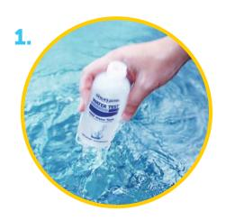
Using a clean plastic cup, collect a water sample from 12"-18" below the surface of your pool.
