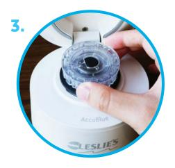
Holding only the sides of the disk, align the D-shape in the disk to the D-shape hub in the test chamber and gently push down.
