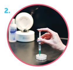
Rinse the syringe before filling for a test. Once filled, and with a new disk on a flat surface, hold syringe vertically to insert the tip into the fill hole.
