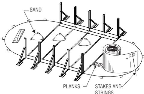
Begin inserting the wall into the bottom tracks in the middle of a bottom plate. At first, the wall is kept in place with one or two stakes and strings (or extra persons). One person uncoils the wall on a beam or a plank, while a second person inserts it in the bottom tracks. Do not uncoil more than 3 m (10') of wall before you install a support bar or stake and string to reinforce the structure.
