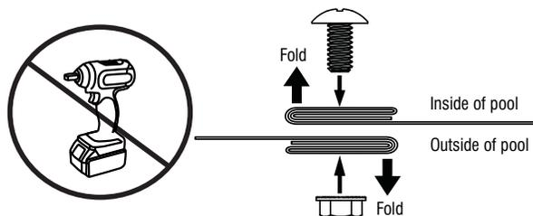
**WARNING:** Never use an impact gun for wall screws. Minimum torque force of 60 inch pounds to maximum of 85 inch pounds.
