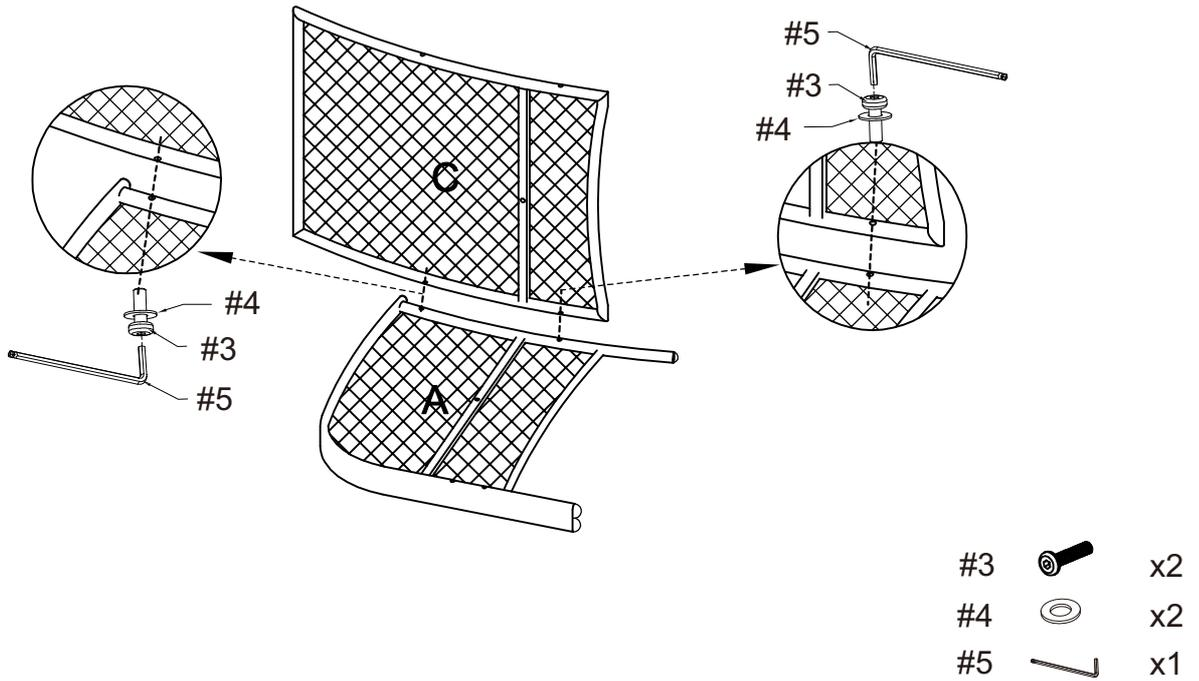
Step 2. Attach seat panel (part D) to left arm panel (part A) and back panel (part C) using medium bolts (part #2), long bolt (part #3), flat washers (part #4) and allen wrench (part #5).
