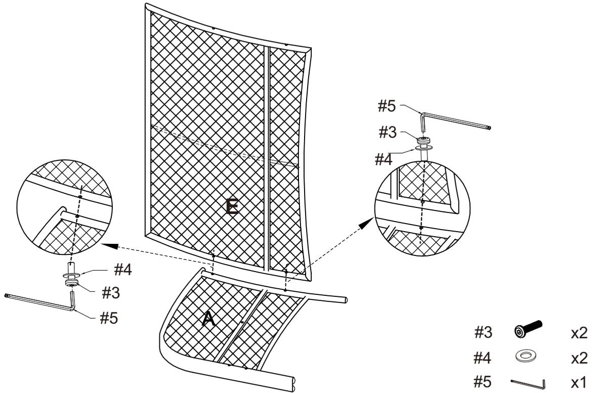
Step 6. Attach seat panel (part F) to left arm panel (part A) and back panel (part E) using medium bolts (part #2), long bolts (part #3), flat washers (part #4) and allen wrench (part #5).
