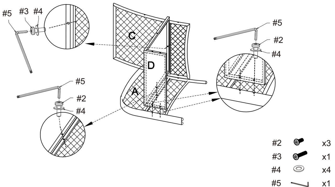
Step 3. Attach right arm panel (part B) to assembled unit (parts A, C & D) using medium bolts (part #2) long bolts (part #3), flat washers (part #4) and allen wrench (part #5).
