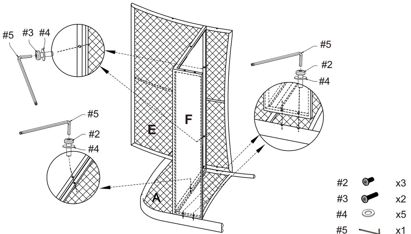
Step 7. Attach right arm panel (part B) to assembled unit (parts A, E & F) using medium bolts (part #2) long bolts (part #3), flat washers (part #4) and allen wrench (part #5).
