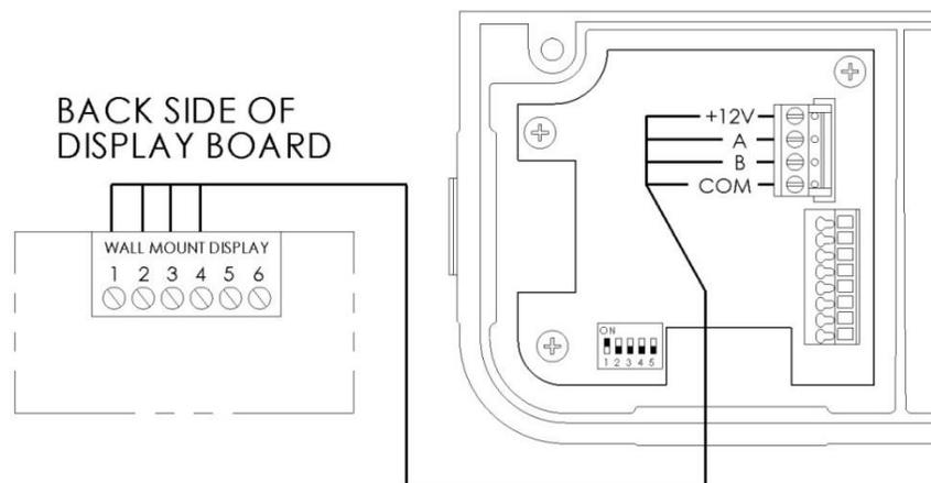
Connection wire must be rated for a minimum of 300V, and may be up to 500 feet in length. Use removable 4-position terminal block connectors for wiring connection to interface and motor drive PCB's taking care to note the wire colors and corresponding numbers next to the connectors. Terminal block must be installed with screws facing up to ensure proper connection. DIP switch #1 must be "ON".
