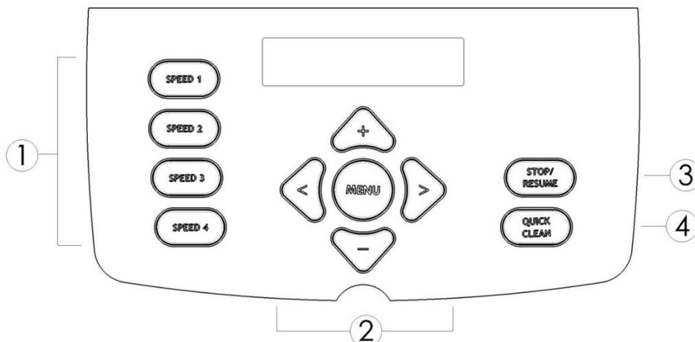
1. **Preset Speeds:** Buttons labeled SPEED 1 thru SPEED 4 can be used to run the pump at a predetermined speed until the next programmed timer is scheduled to begin. Preset Speed settings can be quickly updated using the + and - arrow buttons to change the speed and then pressing the > button to save the new speed setting if desired.
