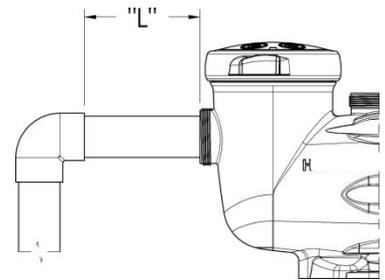
**Note:** It is recommended that a minimum length of straight piping (shown as “L” in above diagram), equivalent to 5 pipe size diameters, be used between the pump suction inlet and any plumbing fittings (elbows, valves, etc.).
