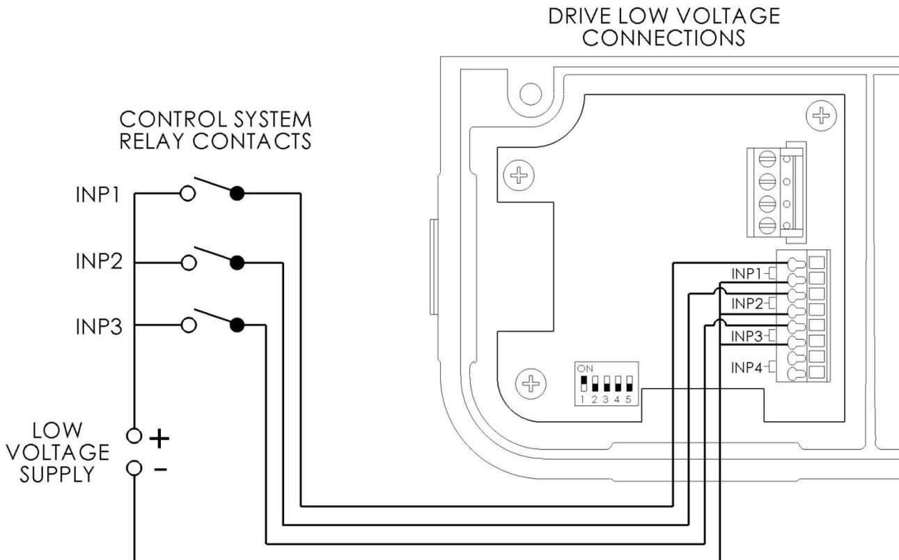
Connection wire must be rated for a minimum of 300V. Inputs are rated to accept a low voltage supply of 18-30 VAC, 9-30 VDC, 50/60 Hz. The "+12V" and "COM" terminals may be used as a low voltage supply, however, these terminals also supply power to the user interface, so care must be taken when connecting to these terminals to ensure proper operation of the user interface. DIP switch #1 must be "ON".
