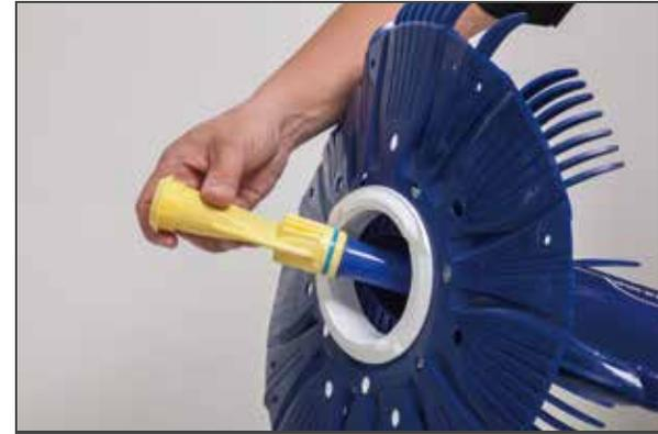
4. If the diaphragm is dirty, but not damaged, clean the valve by rubbing it with a rag under warm water.
