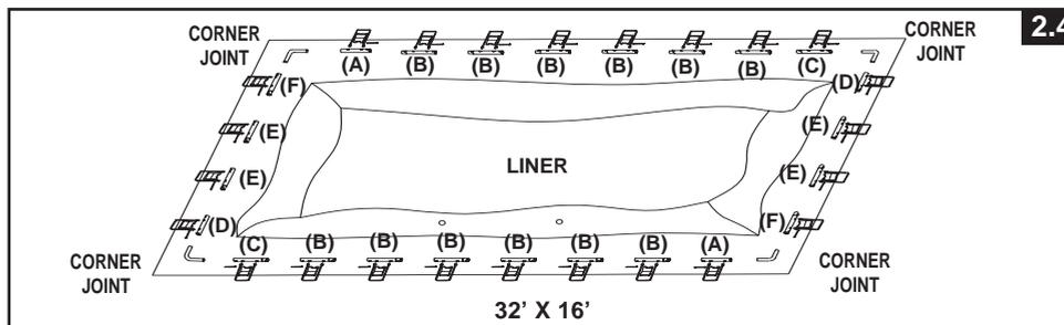
3. Be sure the liner is opened and spread out to its fullest extent on top of the ground cloth. Starting with one side, slide the "A" beams first into the sleeve openings located in each corner. Continue with "B" beam snapping into the "A" beam, and another "C" beam snapping into the "B" beam (see drawing 3).
