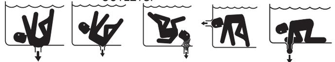
THIS PUMP PRODUCES HIGH LEVELS OF SUCTION AND CREATES A STRONG VACUUM AT THE MAIN DRAIN AT THE BOTTOM OF THE BODY OF WATER. THIS SUCTION IS SO STRONG THAT IT CAN TRAP ADULTS OR CHILDREN UNDER WATER IF THEY COME IN CLOSE PROXIMITY TO A DRAIN OR A LOOSE OR BROKEN DRAIN COVER OR GRATE.
