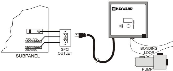
**Bonding:** A lug used for bonding is attached to the bottom of the AquaRite enclosure (see diagram below). The AquaRite must be bonded with an 8 AWG copper wire (6 AWG Canada) to the pool bonding system.
