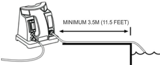
3. Connect the floating cable to the power supply. Use only the original **SharkVAC** Power Supply manufactured by Hayward Pool Products.
