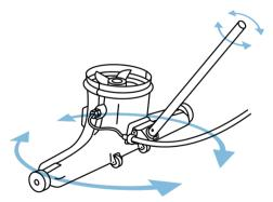
Twist the pole and the vacuum head responds by turning left or right.
