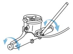
The vacuum head rocks back when you push forward and forward when you pull back, concentrating the suction where it's needed most.
