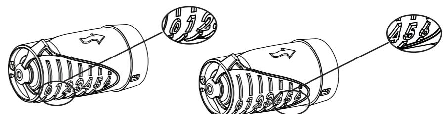
If necessary, adjust FlowKeeper™ Valve (g) setting or adjust valves at the equipment pad.
