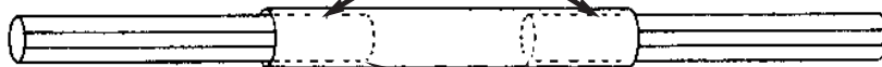
Fig. 3 Insert both end tubes equal distance into center tube and mark on center tube where inner tubes end.
