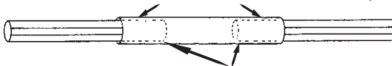
Insert both end tubes equal distance into center tube and mark on center tube where inner tubes end
